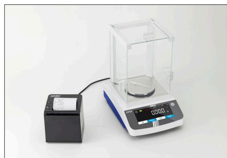
In a GLP-compliant print protocol all weights can be documented, including date, time and identification number.
