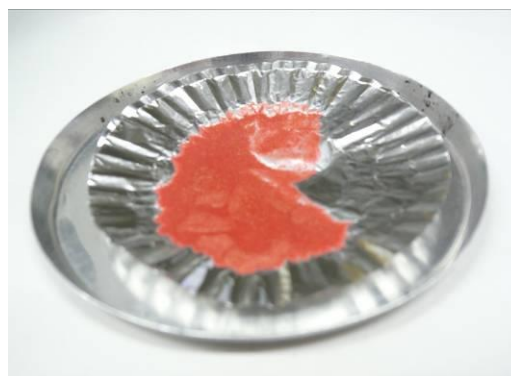
The lip stick melted after 1 min.
