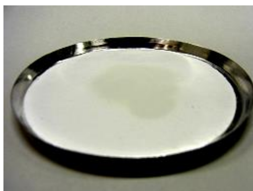
1 g milk distributed evenly via a fiber glass filter
