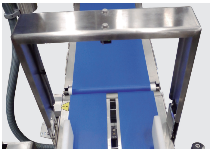
> Detector on arch (horizontal + vertical)
