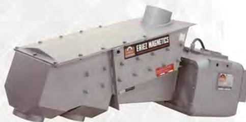
Vibratory sand classifier is used in conjunction with wood fired boiler, to reclaim unburned wood for recirculation through boiler. Screens are used to sift out ash and sand.
