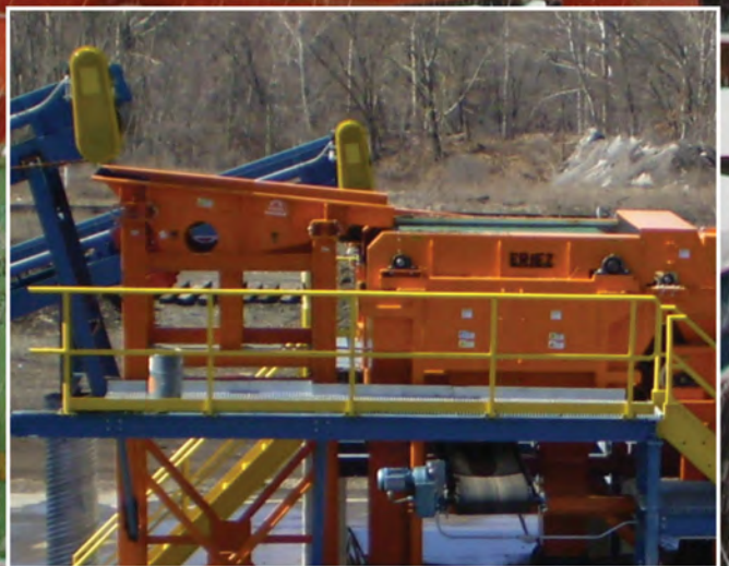
Vibrating action feeds an Eddy Current Separator in a scrap yard.
