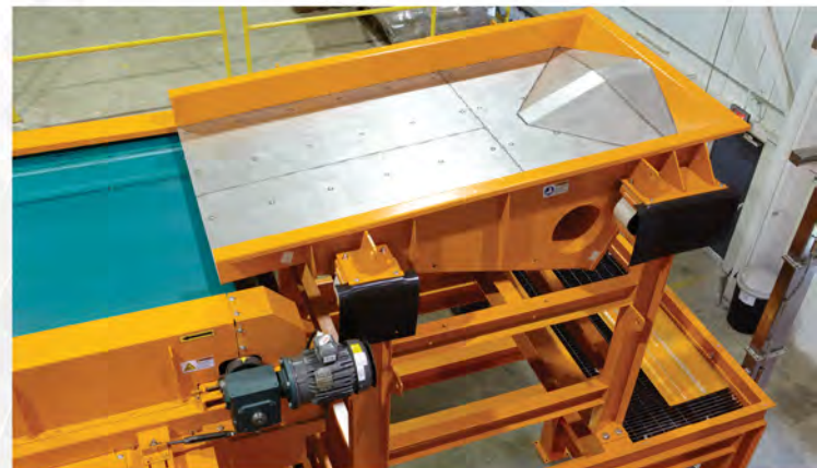
Diversers and liners can improve the spread of material and extend the life of the bed.
