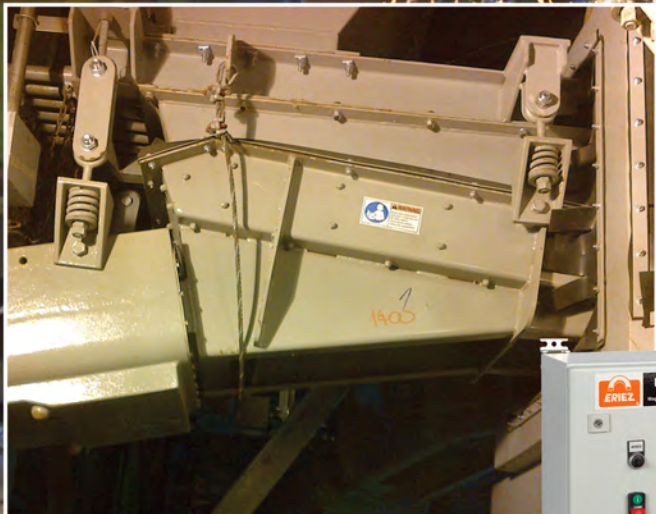
Eriez B-Feeders provide precise control in operations requiring cycling such as a ladle additives system in a steel mill.
