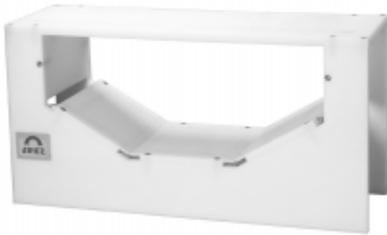
Similar to the Model TR Metalarm, the Model BR Metalarm (bridge design) is excellent for detecting tramp metal in burden depths greater than 14 inches (356 mm). The Model BR Metalarm is available in a series (standard) or transmitter/receiver mode.
