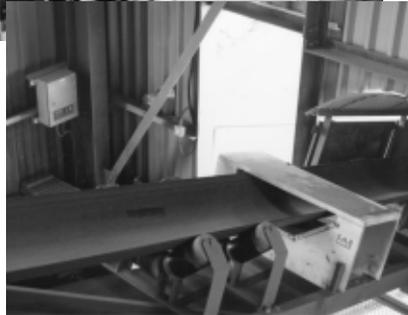
The transmitter/receiver coil combination is excellent for mineralized materials and also for use when nothing smaller than a certain size metal should be detected.
