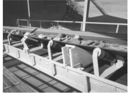
A specialized series of coils is available for situations where idler spacing is unusually close. The Model TR Metalarm is equipped with either a Model 3500 or a Model 3500/QM2 control.
