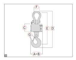
Robust industrial crane scale up to 15 t with radio display and RS-232 data interface for transferring weighing results
