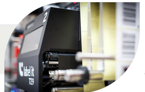
Buffer of labels for high speed application with encoder
