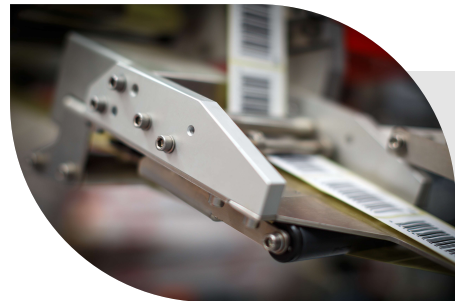
Automatic system for collecting previous label format and preparation of new label format
