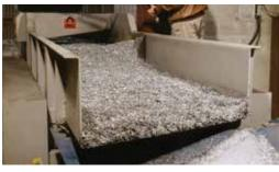
Mechanical Conveyors receive aluminum at a foundry in New York.
