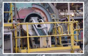
A magnet holds the liner to the drum.
