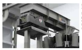
Sanitary Vibratory Feeders present products to weigh scales in packaging applications.
