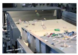
Eddy Current Separator sorts aluminum cans in a recycling facility.
