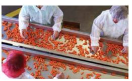
Inspection Conveyor workers visually inspect carrots on sanitary vibratory conveyors.
