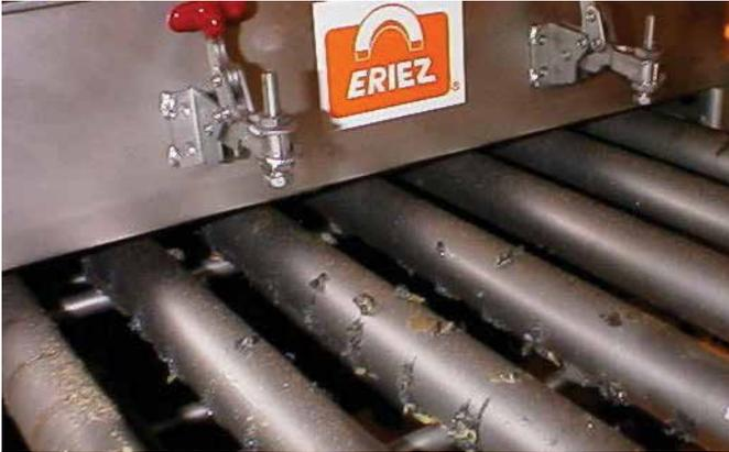
▲ Grain mill uses Xtreme Rare Earth grate magnets to remove metal contaminants.
