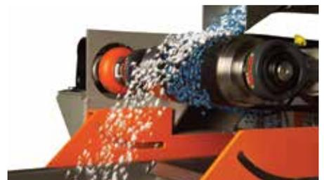
**Magnetic Roll** separates co-molded plastic regrind containing PolyMag™ metallic additive.
