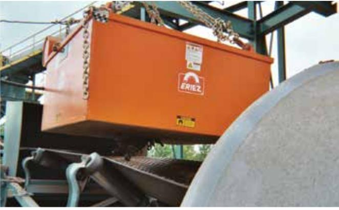
Eriez' origins can be traced back to a single plate magnet installed to remove tramp metals from the flow of grain, thus removing the danger of sparks in the highly flammable environment.
