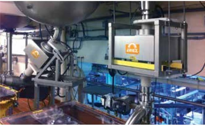
▼ Eriez' Xtreme® Metal Detector is installed in a hot dog packaging plant.
