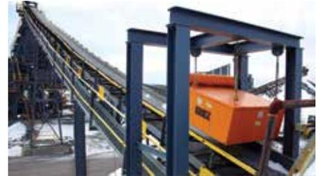
**Suspended Electromagnets** safely and automatically remove tramp iron from heavy product flows such as wood, coal or aggregate being conveyed on belts, vibratory feeders or in chutes.
