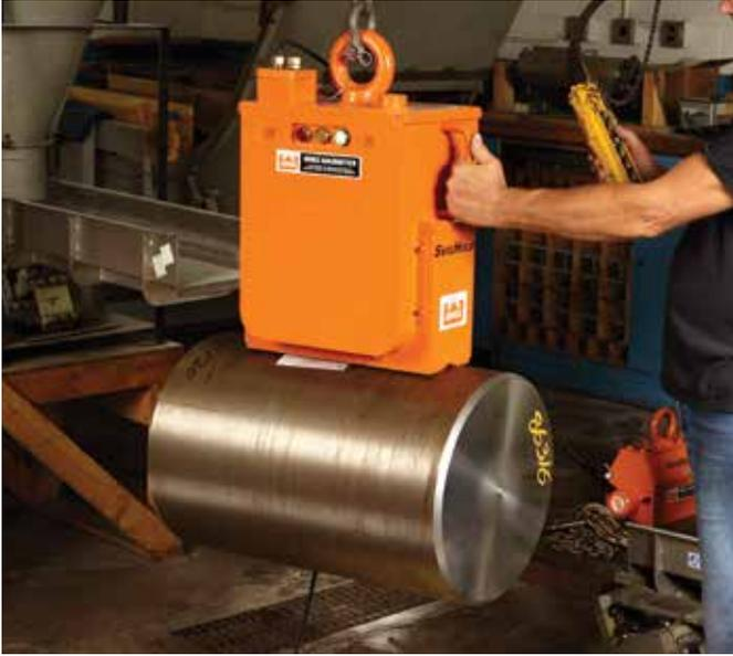
Eriez' SafeHold® Permanent Lift Magnets easily move semi-finished products such as machined parts, castings, press molds, steel plates, bars, tubes and more. These magnets are available in ceramic and rare earth models, lift up to 7,500 pounds with a single magnet, need no costly DC controller, and can be turned on and off with ease.
