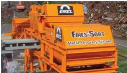
**Finesort®** recovers small ferrous from waste at a scrap yard in Tennessee. Powerful Rare Earth Magnets recover virtually all ferrous metal from crushed automobiles and other scrap.
